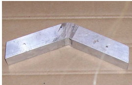
22.5° bracket insert for joining upper panels together
